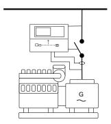
Island mode operation is typically used in power plants that are isolated from the national (or local) electricity distribution network. There are two key types of island mode operation:
