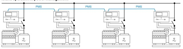
Power plant with synchronising generators. Can also be used in critical power plants with a start signal from an external (ATS) controller.
